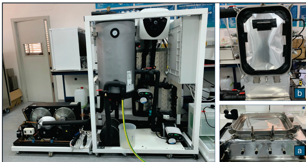
Figure 1. Photograph of the experimental cooling setup left and the prototypes of the tanks: horizontal (a), vertical (b).
