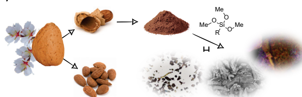
Figure 1. Scheme of the obtention of new biofillers and optical microscope, FESEM and EDX images.
