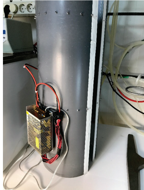
Figure 2.1 Blue LEDs facility built at the University of Almeria for lighting microalgae cultures.
