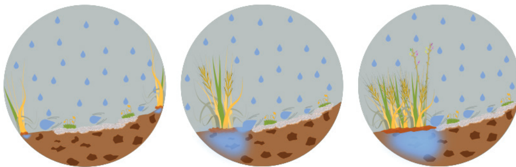
Figure 2. Runoff redistribution process driven by the differences in soil properties between vegetated and surrounding open areas. Open areas have shallow soil with low infiltration rates and are very efficient in runoff generation. Runoff water is infiltrated in the adjacent vegetated patches where soil structure is more developed, and infiltration is favoured. This additional supply of water and nutrients constitute a source of resources for the biotic activity of vegetation and related organisms (e.g., fauna, microfauna, soil microbes, etc) with implications on the ecosystem functioning.
